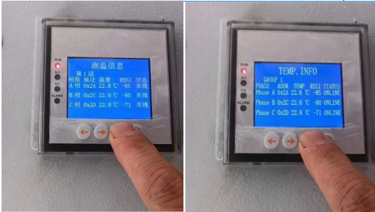
The screen of the Passive Wireless Online Temperature Monitoring System (Multiple language feature is optional for clients)
